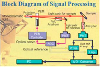
The PEM dual lock-in system of JASCO's ellipsometer provides a stable measurement with additional capabilities including high-speed data sampling and wavelength scanning.
